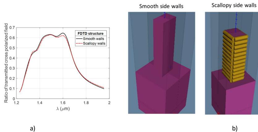
Fig. 1. a) Finite Difference Time Domain Simulations of the ratio of transmitted cross-polarization through the infinite array of identical metamaterial structures. b) The two unit cells considered: One consisting of Si ( $n=3.5$ ) with straight walls, and the other consisting of silicon covered by air-cylinders ( $n=1$ ) in order to mimic the scallop surface resulting from DRIE using the Bosch process.
